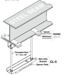
□ Parallel to structural support beams (requires optional 502064 Beam Clamp Kit)
